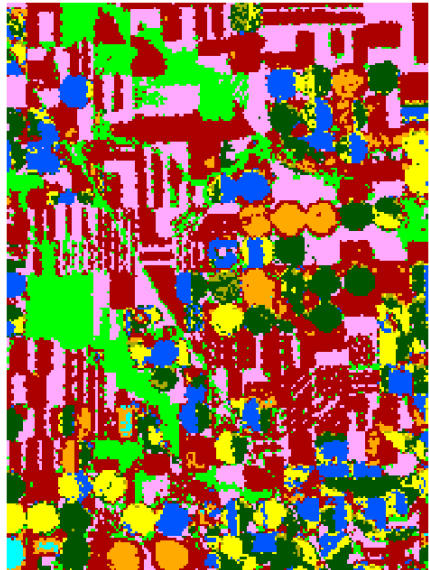
The Maximum Likelihood class raster produced using a priori probabilities has fewer cells assigned to the rare class Potatoes.
