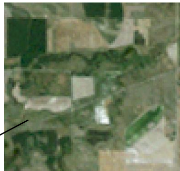
"Natural" color image of the same area for comparison (TM Red, Green and Blue bands assigned to R, G, and B channels, respectively)
