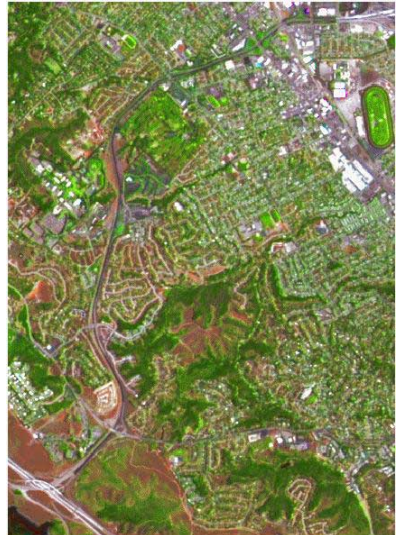
RGBI display of the same three TM rasters with object SPOTPAN as Intensity. The resulting display combines the high spatial resolution of the SPOT panchromatic image with the spectral content of the TM bands.
