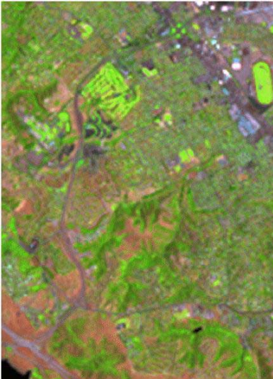
RGB display of objects TM5R , TM4R , and TM3R . (These objects were produced by resampling to the 10-m cell size and extent of the SPOT panchromatic image.)
