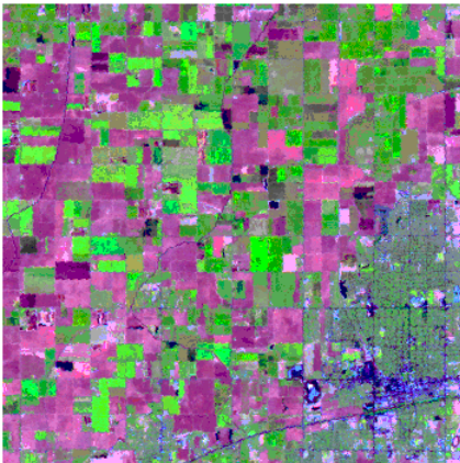
Landsat TM scene for April normalized to June illumination conditions. RGB band assignments are TM5, TM4, and TM3, respectively.
