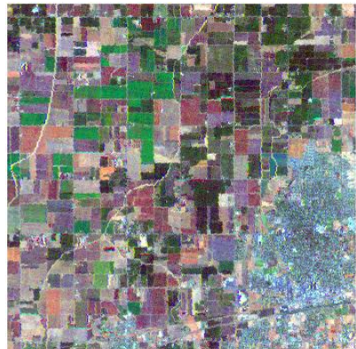
Same band combination after decorrelation stretch. The increased saturation helps distinguish different crops (greens) and different soil types or conditions (shades of orange, red, brown, and lavender).
