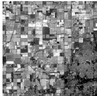
Hanford NDVI image for June 30, 1993. Bright tones indicate fields with actively growing crops.
