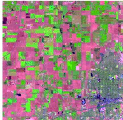
Landsat TM scene of Hanford, CA area for April 27, 1993. TM band 5 (middle infrared) is displayed as red, TM4 (near infrared) as green, and TM3 (red) as blue. Vegetated areas are indicated by green colors and bare soil by pink and magenta.
