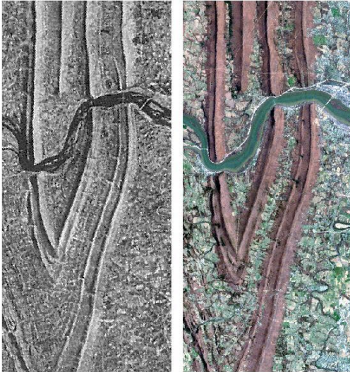
Radar image (left) and reflected light satellite image (right) of the same terrain. Arrow shows radar look direction. Radar image has been projected to ground range (see page 17).
